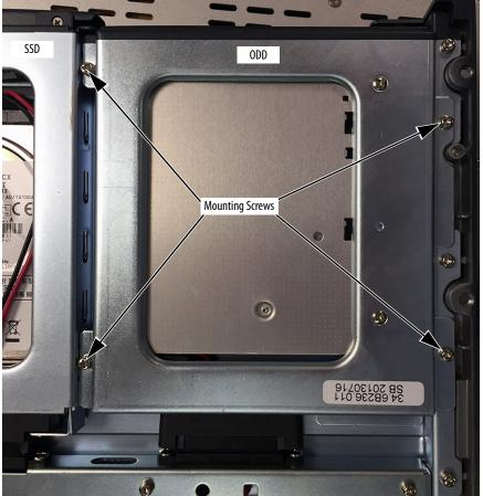
4. Move the loosened ODD until you can access its SATA cable.
